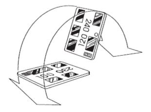
Open cover door and rotate fuse-pull lever to left. Select operating voltage by orienting voltage selection card, desired voltage on top left side. Push card firmly into module slot. Rotate fuse-pull lever back into normal position and re-insert fuse into holders. Use caution in selecting correct fuse value.
